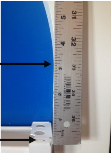
The start of the arch Curve is approx. 3 1/2" above the blind (leg)
